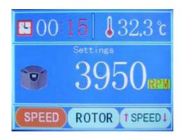
Press the "SET SET" button to enter next step, and the needed hours can be chosen by pressing the "UP" or "DOWN" button.
