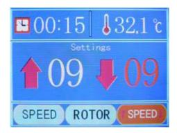
UP" button to adjust the acceleration of the rotating speed, or touch the screen and click the icon to do the same operation. There are 10 acceleration levels: 0 is the slowest while 9 is the fastest.
