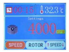
Press the " UP" or " DOWN" button to adjust the rotating speed value.
