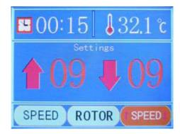
DOWN" button to adjust the deceleration of the rotating speed, or touch the screen and click the icon to do the same operation. There are 10 deceleration levels: 0 is the slowest while 9 is the fastest.
