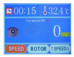
2) Press the "SET" button to enter the first adjustment panel, or touch the screen and click the rotating speed area to enter the same panel.
