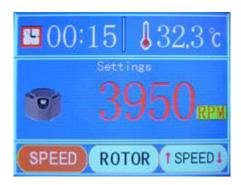
• Press the "SET" button to enter the rotating speed adjustment panel. Next, press the "UP" or "DOWN" button and press the "SET" button again to enter the time adjustment area. The needed minutes can be chosen by pressing the "UP" or "DOWN" button.
